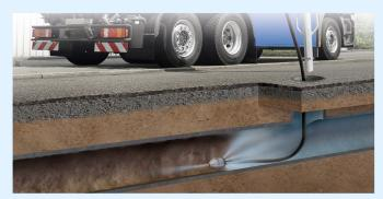
Sewer cleaning and inspections are essential to maintaining a properly functioning system and extending it's life cycle. It is the first step in determining both the condition of infrastructure and if any repairs are needed. We recommend televising roughly 20% of your sewer system each year as part of a regular maintenance and protection plan.
